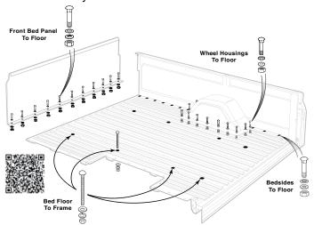
Bed Floor Hardware Kit includes the hardware to attach the front bed panel, bedsides and the wheel housings to the bed floor. Bed to frame mounting kit is also included. Fits trucks with stock wheel housings only. 1 kit required per vehicle.
