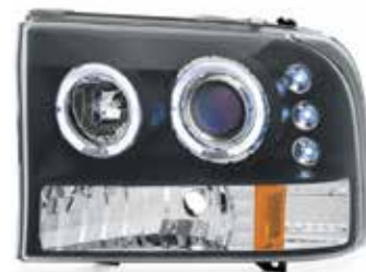
42-1617 One-piece assembly to replace the OE two-piece Headlight/Parklight.
